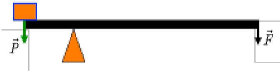
$$F \times d = P \times d \quad 500 \times 20 = F \times 80 \quad 10000 = F \times 80 \quad F = 10000/80 \quad F = 125 \text{ N}$$
